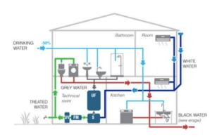
Figure 22: Greywater reuse at building level<sup>43</sup>
