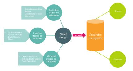
Figure 19: Conceptual view of the anaerobic digestion of the organic fraction of the MSW<sup>38</sup>
