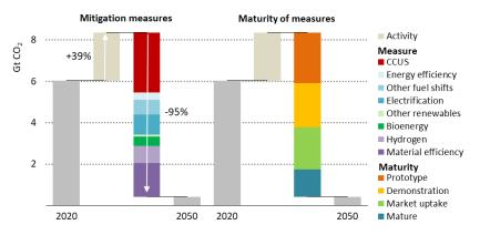
Figure 16: Global CO<sub>2</sub> emissions in heavy industry and reductions by mitigation measure and technology maturity category in the Net-Zero Emissions by 2050 Scenario<sup>24</sup>
