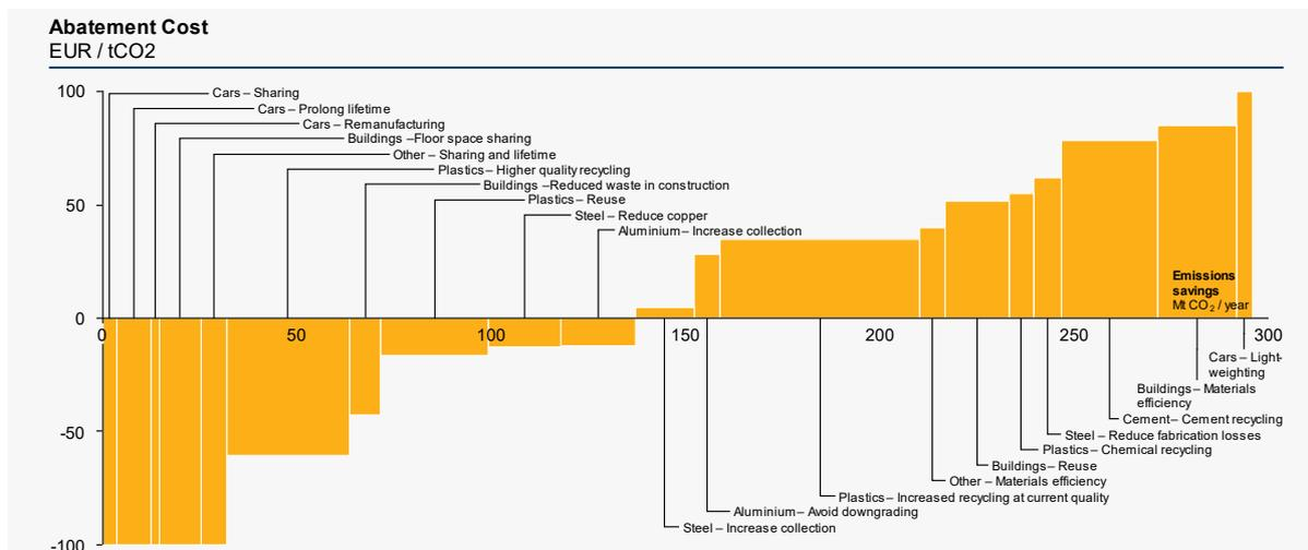
Figure 36: A first abatement cost curve for circular solutions – much of the potential is cost-effective<sup>58</sup>
