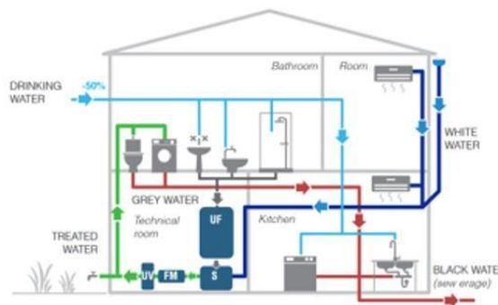
Figure 22: Greywater reuse at building level<sup>43</sup>
